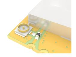
0R resistance welding as shown in the above picture(left), connector type of antennas is stamp hole. Users need to change the 0R resistance as the above picture(right) if want the antennas types as IPEX.
