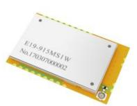
E19-915MS1W is a 1W wireless transceiver module, operates at 915MHz with SPI RF interface. It 's small-sized SMD module with low-noise amplifier to enhance the sensitivity. With stable batch production, the module is suitable for various applications.
