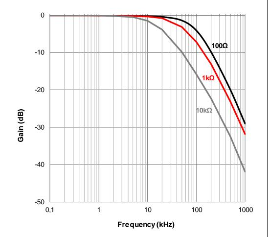
Testcondition:  $I_C = 2mA$ ;  $V_{CE} = 2V$ ; TA= 25°C
