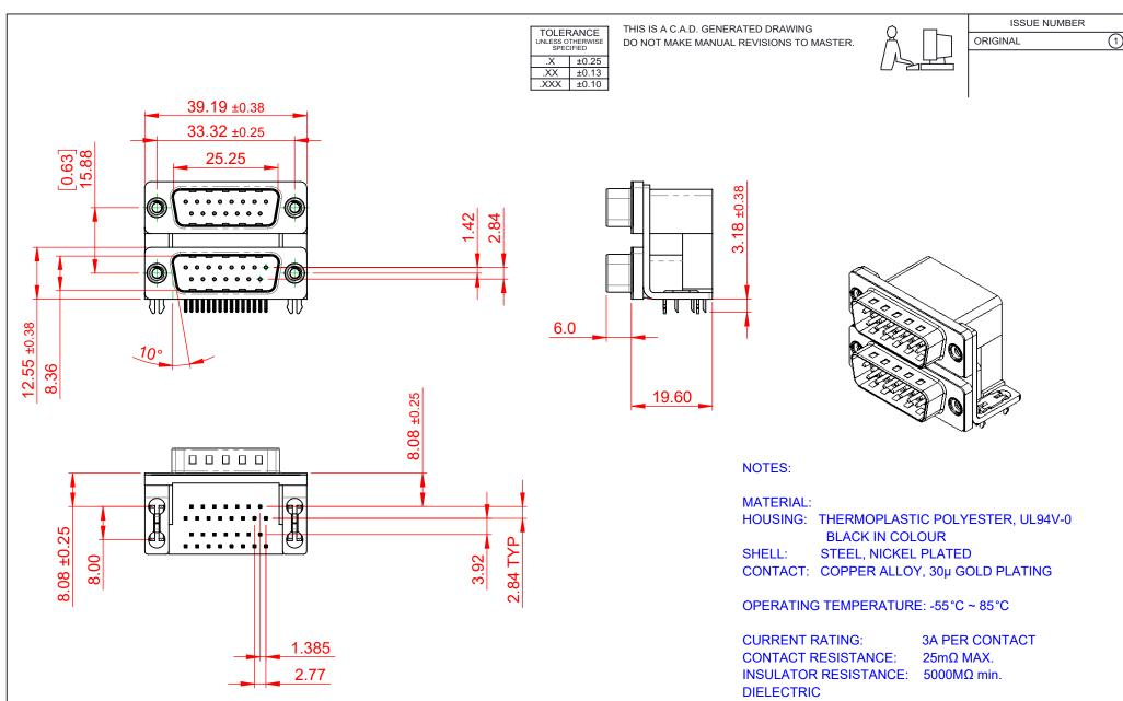
WITHSTANDING VOLTAGE: 1000V AC rms
