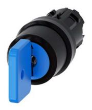
Key-operated switch O.M.R, 22 mm, round, plastic, lock number 73038, blue, with 2 keys, 3 switch positions I-O<II, left latching, right momentary contact type, actuating angle  $2x45^{\circ}$ , 10:30h/12h/13:30h, Key removal O Z=50-unit packaging
