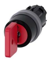
Key-operated switch O.M.R, 22 mm, round, plastic with metal front ring, lock number 73037, red, with 2 keys, 3 switch positions I-O-II, latching, actuating angle 2x45°, 10:30h/12h/13:30h, key removal O, with laser labeling, upper case and lower case, always upper case at beginning of line
