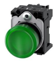
Indicator lights, 22 mm, round, plastic, green, lens, smooth, with holder, LED module, with integrated LED 230 V AC, screw terminal, with laser labeling, symbol number according to, ISO 7000 or IEC 60417
