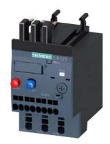
Overload relay 0.14...0.20 A Thermal For motor protection Size S00, Class 10 Contactor mounting Main circuit: Spring-type terminal Auxiliary circuit: spring-type terminal Manual-Automatic-Reset
