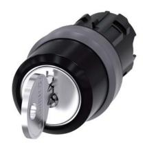
RONIS key-operated switch, 22 mm, round, plastic with metal front ring, lock number SB30, with 2 keys, 3 switch positions I-O-II, latching, actuating angle 2x45°, 10:30h/12h/13:30h, Key removal II, possible special locks: SB31, 421, 455, with laser labeling, upper case
