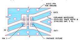
1. TRACE WIDTH AND GAP PARAMETERS ARE SHOWN FOR ROGERS RO4350B WITH DIELECTRIC THICKNESS .010°±.011°. COPPER: 1/2 0Z. EACH SIDE. FOR OTHER MATERIALS TRACE WIDTH AND GAP MAY NEED TO BE MODIFIED.
