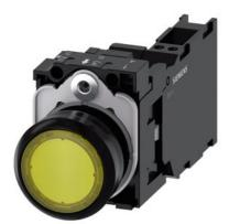
Illuminated pushbutton, 22 mm, round, plastic, yellow, pushbutton, flat, momentary contact type, with holder, 1 NO+1 NC, LED module with integrated LED 24 V AC/DC, Spring-type terminal
