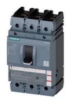
circuit breaker 3VA5 UL frame 250 breaking capacity class M 35kA @ 480 V 3-pole, line protection TM210, FTFM, In=70A overload protection Ir=70A fixed short-circuit protection Ii=10 x In UL489 SB (naval), 50 deg. cel. nut keeper kit on both sides
