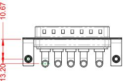
POWER/CO-AX CONTACT RATING: (IF PRESENT) SIGNAL CONTACT CURRENT RATING: 5A PER CONTACT SIGNAL CONTACT RESISTANCE:  $10m\Omega$  MAX.
