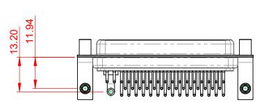
THERMOPLASTIC POLYESTER, UL94V-0 STEEL, NICKEL PLATED COPPER ALLOY, 30µ GOLD PLATED
