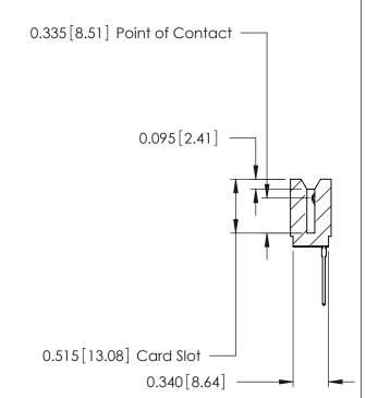
746 Series Ultra-Mate Card Edge Connector - Press Fit
