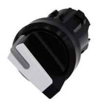
Selector switch, illuminable, 22 mm, round, plastic, white, selector switch, short, 2 switch positions O-I, latching, actuating angle 90°, 10:30h/13:30h, with laser labeling, lower case
