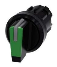
Selector switch, illuminable, 22 mm, round, plastic, green, selector switch, short, 3 switch positions I>O<II, momentary contact on the left, latching on the right, actuating angle  $2x45^{\circ}$ , 10:30h/12h/13:30h, with laser labeling, upper case
