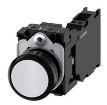
Pushbutton, 22 mm, round, plastic, white, pushbutton, flat, momentary contact type, with holder 1 NO+1 NC, spring-type terminal, with laser labeling, upper case and lower case, always upper case at beginning of line
