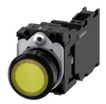
Illuminated pushbutton, 22 mm, round, plastic, yellow, pushbutton, flat, momentary contact type, with holder, 1 NO+1 NC, LED module with integrated LED 110 V AC, spring-type terminal, with laser labeling, upper case
