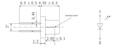
all dimensions in mm. Tolerance  $\pm$  0, 2 except given ones \* at the bottom of the LED
