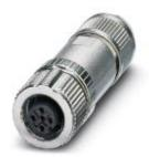
Connector, 4-position, shielded, Socket straight M12 SPEEDCON, A-coded, Spring-cage connection, knurl material: Zinc die-cast, nickel-plated, external cable diameter 4 mm ... 8 mm
