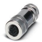
Bus system connector, CAN Bus/DeviceNet, 5-position, shielded, Socket straight M12, A-coded, Screw connection, knurl material: Zinc die-cast, nickel-plated, cable gland Pg9, external cable diameter 6.5 mm ... 8.5 mm
