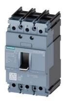
circuit breaker 3VA5 UL frame 125 breaking capacity class H 65kA @ 480 V 3-pole, line protection TM210, FTFM, In=20A overload protection Ir=20A fixed short-circuit protection Ii=15 x In UL489 SB (naval), 50 deg. cel. cable connection on both sides
