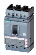
circuit breaker 3VA5 UL frame 250 breaking capacity class H 65kA @ 480 V 3-pole, line protection TM230, FTAM, In=200A overload protection Ir=200A fixed short-circuit protection Ii=5...10 x In UL489 SB (naval), 50 deg. cel. cable connection on both sides
