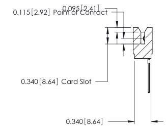
ACAD REFERENCE NO. 746 Series Ultra-Mate Card Edge Connector - Press Fit DRAWN: Part Number: 746-025-553-506 CHECKED: **EDAC INC** THESE DRAWINGS AND SPECIFICATIONS ARE THE PROPERTY OF EDAC INC.,AND TORONTO, ONTARIO SHALL NOT BE REPRODUCED, OR COPIED CANADA OR USED AS THE BASIS FOR THE MANUFACTURE OR SALE OF APPARATUS
