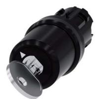
key-operated switch Siemens, 22 mm, round, plastic, lock number SSG10, with 2 keys, 2 switch positions O-I, latching, actuating angle 90°, 10:30h/13:30h, key removal I, with laser labeling, upper case
