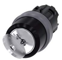
RONIS key-operated switch, 22 mm, round, plastic with metal front ring, lock number SB30, with 2 keys, 2 switch positions O-I, latching, actuating angle 90°, 10:30h/13:30h, key removal O+I, possible special locks: SB31, 421, 455, with laser labeling, upper case
