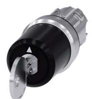
key-operated switch Siemens, 22 mm, round, metal, shiny, lock number SSG10, with 2 keys, 3 switch positions I-O-II, latching, actuating angle 2x45°, 10:30h/12h/13:30h, key removal II, with laser labeling, inscription or symbol customer-specific selection with SIRIUS ACT configurator (CIN)
