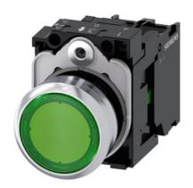
Illuminated pushbutton, 22 mm, round, metal, shiny, green, pushbutton, flat, momentary contact type, with holder, 1NO, LED module with integrated LED 110 V AC, screw terminal, Z=20-unit packaging
