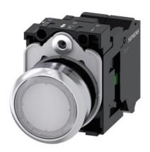
Illuminated pushbutton, 22 mm, round, Metal, shiny, white, pushbutton, flat, momentary contact type, with holder, 1NO, LED module with integrated LED 230 V AC, spring-type terminal, with laser labeling, upper case and lower case, always upper case at the beginning of the word
