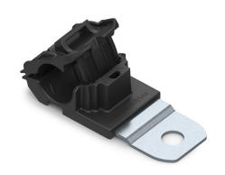
Ratchet P-Clamp, 0.50 - 0.77" Bundle Dia, 180° Short, 0.33" Hole Dia, PA66HIRHSUV/ST/ZN, Black, 20/bag
