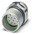
Device connector for front wall, straight, shielded: yes, for standard and SPEEDCON interlock, M23, No. of pos.: 16, type of contact: Socket, Solder connection, Axial seal, Central fastening M20 x 1.5, can be positioned via a locking nut
