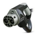
DC charging cable, DC charging cable with Vehicle Connector, open cable end, with protective cap, GB/T, GB/T 20234.3-2015, 125 A / 750 V (DC), design line Standard, cable: 8 m, black, straight, NOTE: Cable management may be required., mating face: gray, handle area: gray
