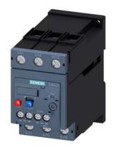
Overload relay 54...65 A Thermal For motor protection Size S2, Class 10 Stand-alone installation Main circuit: Screw Auxiliary circuit: Screw Manual-Automatic-Reset
