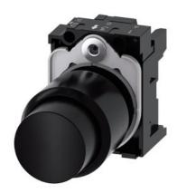
Pushbutton, compact, with extended stroke (12 mm), 22 mm, round, plastic, black, pushbutton, raised, momentary contact type, with holder
