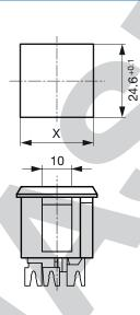
Panel thickness X 0.8 - 1.2 mm: 24.6 mm 1.3 - 1.6 mm: 24.8 mm
