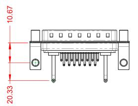
POWER/CO-AX CONTACT RATING: (IF PRESENT) SIGNAL CONTACT CURRENT RATING: 5A PER CONTACT SIGNAL CONTACT RESISTANCE:  $10m\Omega$  MAX. **INSULATOR RESISTANCE:**
