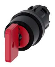
Key-operated switch O.M.R, 22 mm, round, plastic, lock number 73037, red, with 2 keys, 3 switch positions I>O<II, momentary contact type, actuating angle 2x45°, 10:30h/12h/13:30h, key removal O, with laser labeling, upper case
