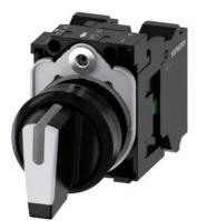
Selector switch, illuminable, 22 mm, round, plastic, white, selector switch, short, 3 switch positions I>O<II, momentary contact type, 10:30h/12h/13:30h, with holder, 1 NO, 1 NO, spring-type terminal, with laser labeling, lower case
