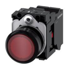
Illuminated pushbutton, 22 mm, round, plastic, red, pushbutton, flat, momentary contact type, with holder, 1NC, LED module with integrated LED 24 V AC/DC, spring-type terminal, with laser labeling, inscription or symbol Customer-specific selection with SIRIUS ACT configurator (CIN)
