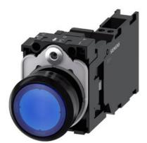
Illuminated pushbutton, 22 mm, round, plastic, blue, pushbutton, flat, momentary contact type, with holder, 1 NO+1 NC, LED module with integrated LED 110 V AC, spring-type terminal, with laser labeling, upper case and lower case, always upper case at beginning of line
