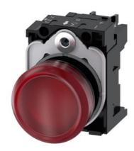
Indicator lights, 22 mm, round, plastic, red, lens, smooth, with holder, LED module with integrated LED 110 V AC, screw terminal, with laser labeling, symbol number according to, ISO 7000 or IEC 60417
