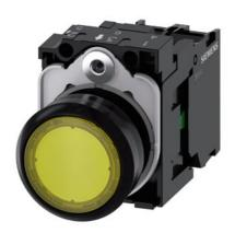
Illuminated pushbutton, 22 mm, round, plastic, yellow, pushbutton, flat, momentary contact type, with holder, 1NO, LED module with integrated LED 24 V AC/DC, screw terminal, with laser labeling, upper case and lower case, always upper case at beginning of line
