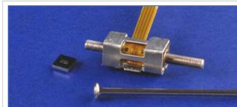
**SQUIGGLE RV motor and driver** inside every M3-L module: the world's smallest linear motor system.
