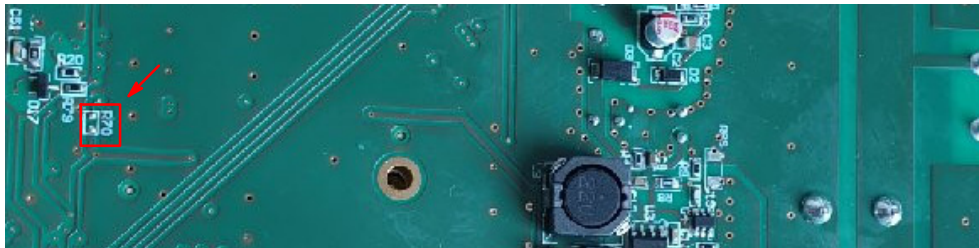
Figure 10. UCB UART Disable via Soldering R70 at MDK Board
