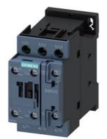
power contactor, AC-3 17 A, 7.5 kW / 400 V 1 NO + 1 NC, 400 V AC, 50 Hz, 400-440 V, 60 Hz, 3-pole, Size S0, screw terminal
