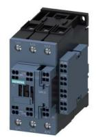
power contactor, AC-3 51 A, 22 kW / 400 V 2 NO + 2 NC, 230 V AC, 50 Hz 3-pole, size S2, spring-loaded terminal lateral auxiliary switch block
