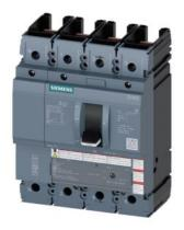
Circuit breaker 3VA5 UL Frame 250 Breaking capacity class C 100kA @ 480 V 4-pole, line protection TM210, FTFM, In=50A Overload protection Ir=50A fixed Short-circuit protection Ii=10 x In N conductor Unprotected Without connection
