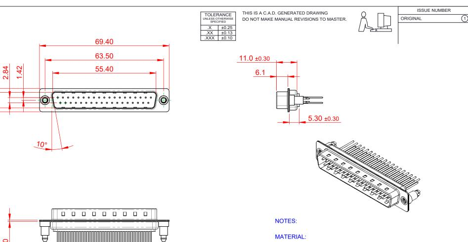
HOUSING: WHITE THERMOPLASTIC POLYESTER, UL94V-0 STEEL, TIN PLATED SHELL: CONTACT: COPPER ALLOY, 15µ GOLD PLATED
