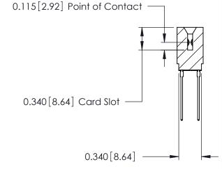
ACAD REFERENCE NO. 746 Series Ultra-Mate Card Edge Connector - Press Fit DRAWN: J.LEE Part Number: 746-024-541-601 CHECKED: **EDAC INC** SCALE: THESE DRAWINGS AND SPECIFICATIONS ARE THE PROPERTY OF EDAC INC.,AND TORONTO, ONTARIO SHALL NOT BE REPRODUCED, OR COPIED CANADA OR USED AS THE BASIS FOR THE MANUFACTURE OR SALE OF APPARATUS YOUR CONNECTION TO QUALITY & SERVICE WITHOUT WRITTEN PERMISSION.
