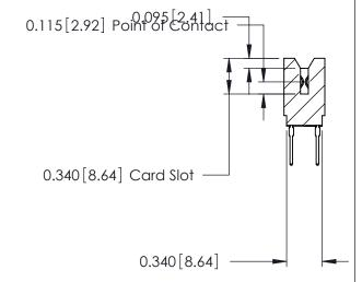
ACAD REFERENCE NO. 746 Series Ultra-Mate Card Edge Connector - Press Fit DRAWN: Part Number: 746-072-527-606 CHECKED: **EDAC INC** THESE DRAWINGS AND SPECIFICATIONS ARE THE PROPERTY OF EDAC INC.,AND TORONTO, ONTARIO SHALL NOT BE REPRODUCED, OR COPIED CANADA OR USED AS THE BASIS FOR THE
